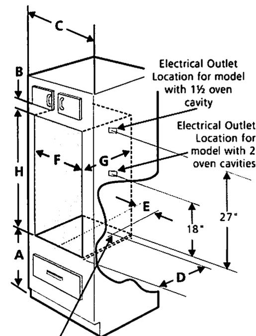
Drill a 1/2" diameter hole for gas hook up
