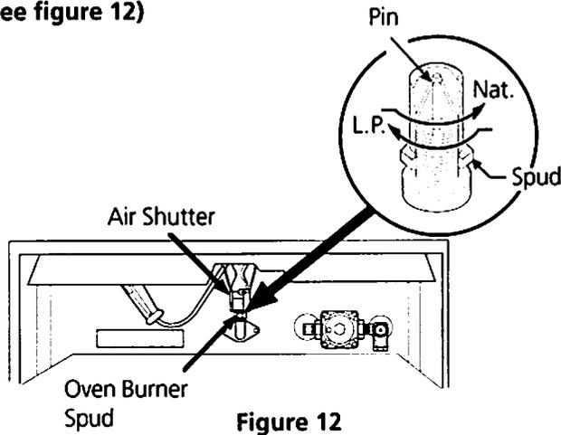
Using a 1/2" wrench, turn down the adjustable spud which injects gas into the oven burner. Spud approximately 2 1/2 turns until snug against the LP metering pin. Do not overtighten (see figure 12).
