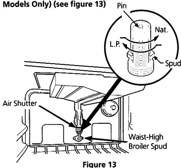
Using a 1/2" wrench, turn down the adjustable spud which injects gas into the oven burner. Spud approximately 2 1/2 turns until snug against the LP metering pin. Do not overtighten (see figure 13).
